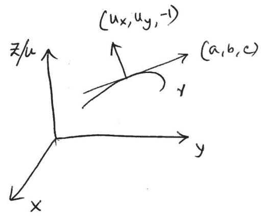
If  $\gamma(t) = (x(t), y(t), z(t))$  is a characteristic curve then the tangent vector is  $(\frac{dx}{dt}, \frac{dy}{dt}, \frac{dz}{dt})$ , which is by definition:
